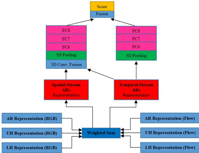
Fig. 5. Using the TS-Net2 for explanation (with the VGG16 architecture). Illustrations of 1) the combination of the feature maps of 3 actor-related regions (ARs: AR, UH, LH) at the last convolutional layer (Conv5\_3) and, 2) the fusion of spatial stream and temporal stream via the ST-CF operation.
