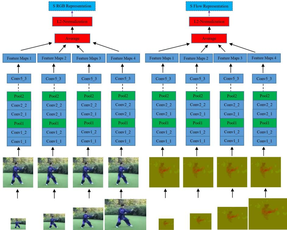
Fig. 4. Using **scene** (S) for explanation (on the TS-Net1) of multi-scale based data augmentation operation. Fusing multi-scale feature representations of one input semantic cue to form the final feature representation in the spatial-stream (e.g., S RGB representation) and the temporal-stream (e.g., S Flow representation) at the last convolutional layer (Conv5\_3) of VGG16 model.
