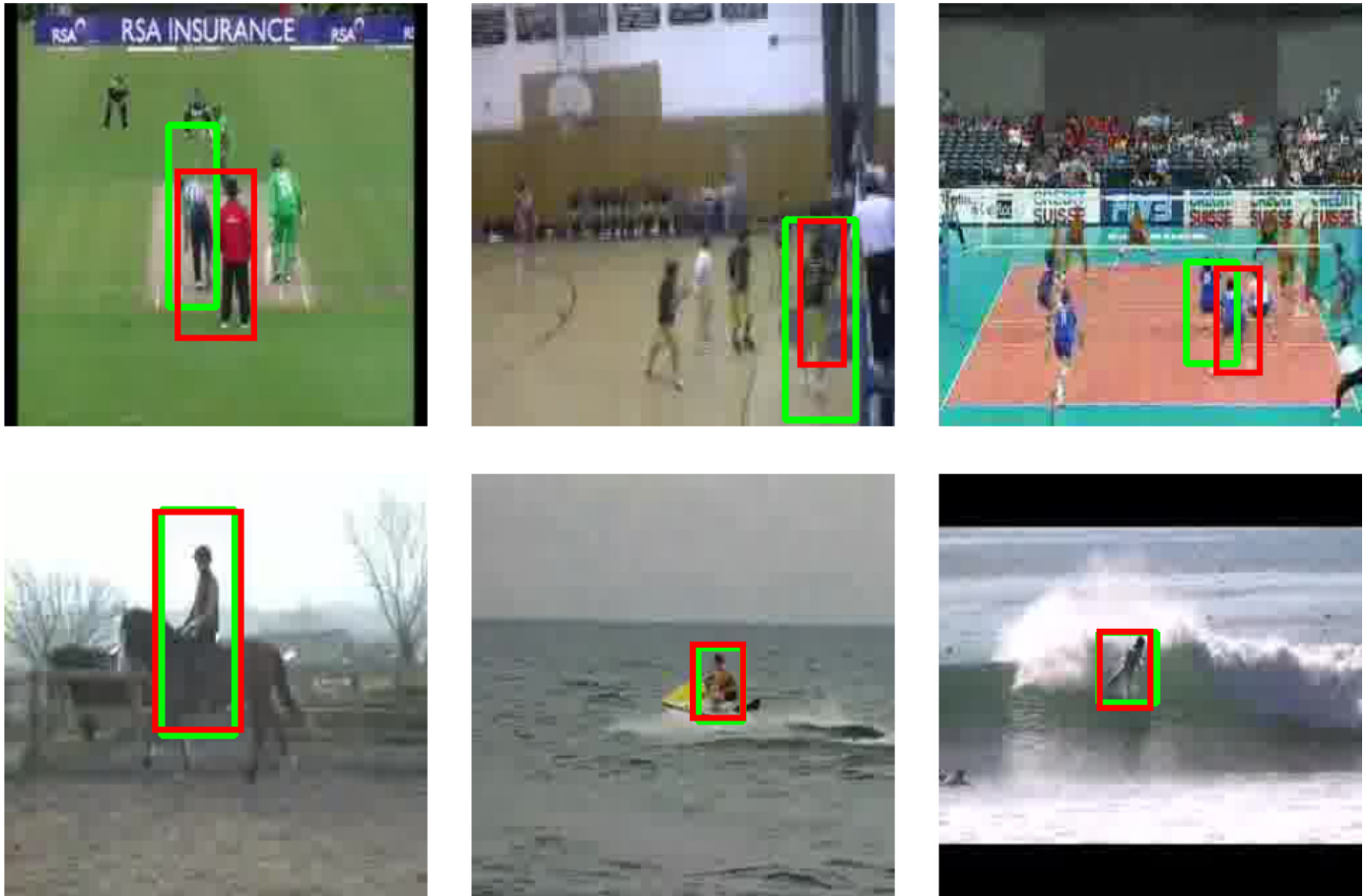
Fig. 5. Examples of regressed bounding boxes (red) and the ground truth (green). We can find our model have a bad performance on the Scenarios that contain multiple people. But our model have good regression performance in single person scene.
